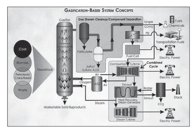
The heart of gasification-based systems is the gasifier. A gasifier converts hydrocarbon feedstock into gaseous components by applying heat under pressure in the presence of steam.
